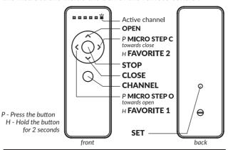
In order for a remote control to execute commands on a motor, its active channel must be paired with that motor. See topic "Pairing Process" for instructions.
