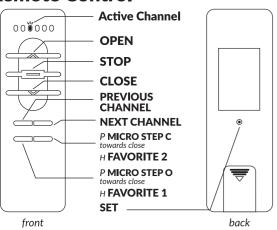
P - Press the button H - Hold the button for 2 seconds
