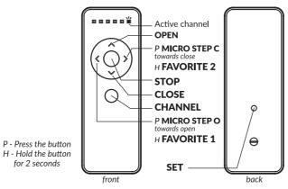
For a remote control to execute commands on a motor. its active channel must be paired with that motor. Refer to the "Pairing Process" section for instructions.
